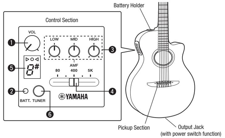
The built-in preamplifier is automatically turned ON when a guitar cable is connected to the output jack. The tuner can be turned on or off anytime.
