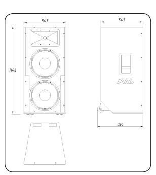
Ultimate frontal full-range system with significant power capacity and high sensitivity. Based on two high-power 15" woofers and 2" throat diameter 4" voice coil HF driver, Top 550 offers greatest sonic performance possible horn systems notwithstanding. Provided with transportation friendly castor wheels for convenience, Top 550 is great for fixed high profile installations, as a backline or FOH speaker.
